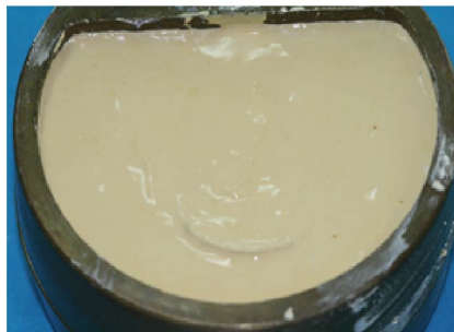
Do 2nd investing around inside teeth and invest up to flask.
