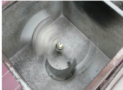
Casting Casting using centrifugal casting machine
